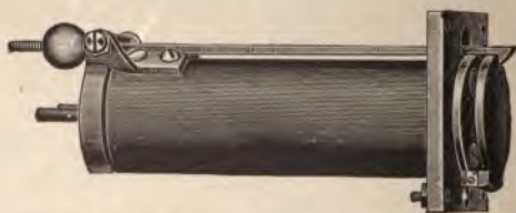
FIG. 117.—Tubular Drop of the Couch & Seeley Co. The tube is drilled from a solid rod of iron, and by the attachment of the magnet core gives a double-pole effect at the armature. Connections of the night bell circuit are shown beneath the hinge of the shutter.
